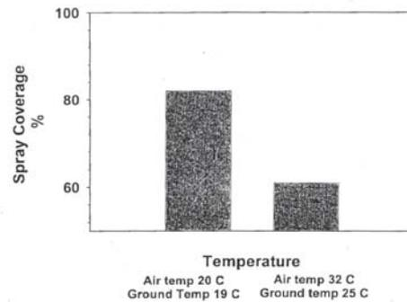
**Figure 2.** Boom spray coverage at two temperatures (Source A. Storrie, NSW DPI)
