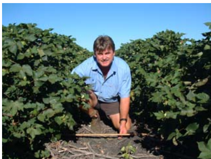
Brad Tatzenko of Tatzenko Consultancies measuring a furrow profile for one of his clients as part of a Surface Irrigation Evaluation
